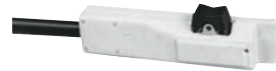
RMLS-14 (14-pin plug) 129337 Momentary- and maintained-contact rocker switch for contacter control. Push forward for maintained contact and backward for momentary contact. Includes 26.5-foot (8 m) cord with plug.
