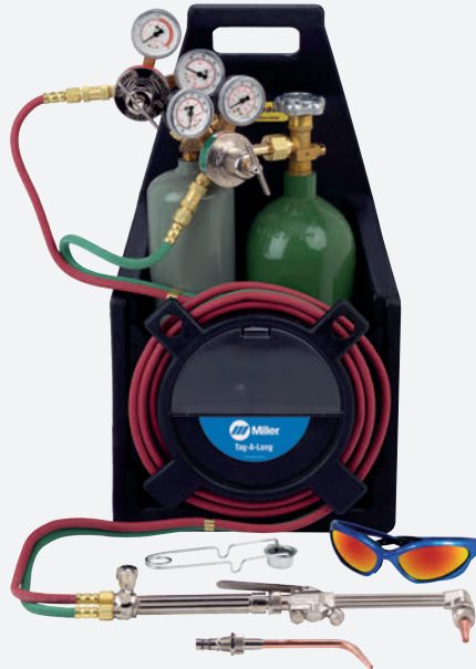
TL-550 (Tag-A-Long) includes portable carrier for 10–20 cu. ft. cylinders.
